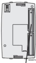
Turn thermostat over, insert fresh AAA alkaline batteries, then reinstall thermostat.
