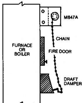
**Fig. 3. Chain linkage arrangement.**
