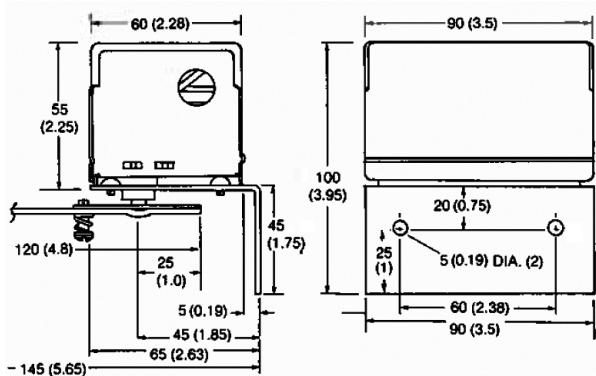
**Fig. 2. Short Bracket Model with arm linkage attached.**
