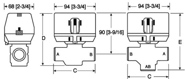
Fig. 1. Nominal Dimensions in inches and millimeters
