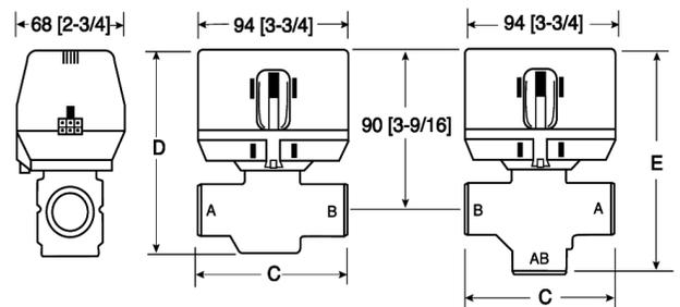
Fig. 1. Nominal dimensions in inches [millimeters]
