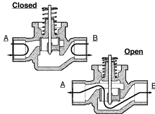
**Fig. 2. Fluid Flow of 2-way valves**
