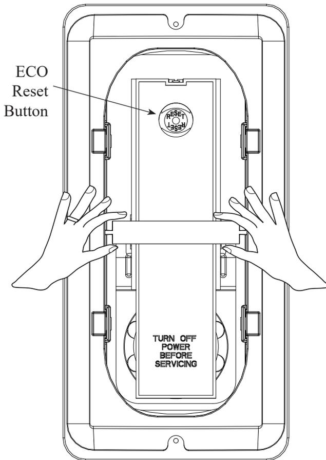
In order to replace the ECO,thermistor or heating element, remove the cavity insert crossbar by following the instructions below:
