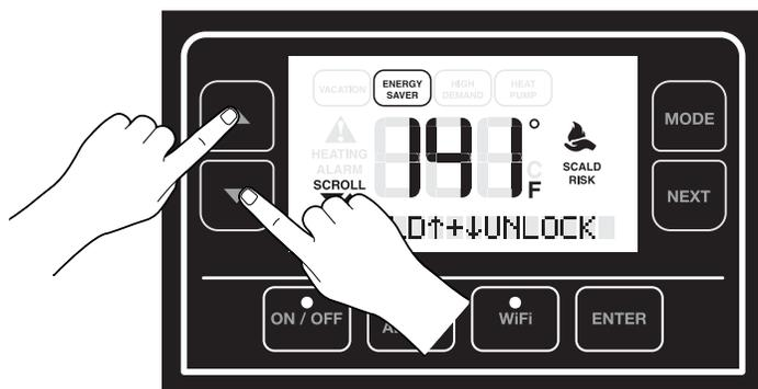
**Enable** high temperatures (+140°) by pressing and holding both "UP" and "DOWN" buttons for 3 seconds when temperature is set to 140°F.
