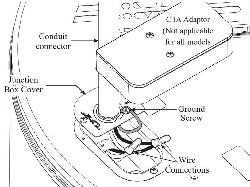
**A separate branch circuit with copper conductors, overcurrent protective device and suitable disconnecting means must be provided by a qualified electrician.**
