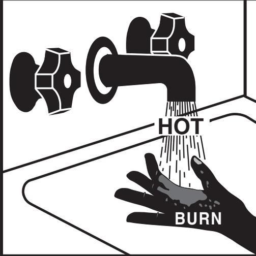
**Water temperature over 125°F (52°C) can cause severe burns instantly or death from scalds.**
