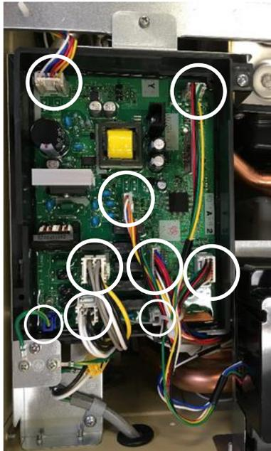
2. Remove top center screw from control boardmounting bracket, and 2 screws located on bottom.
