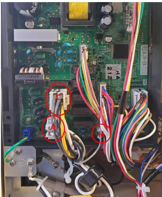
3. Shift the control board and locate total of four (4) Molex connectors; one (1) blue, one (1) yellow, two (2) white behind the control board.
