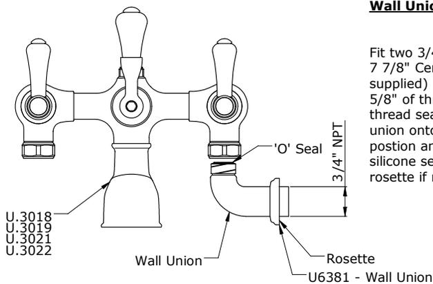
Fit two 3/4" NPT female fittings into the wall at 7 7/8" Centers. Fit a 3/4" NPT male shank (not supplied) into the fitting so that no more than 5/8" of thread is protruding from the wall. Apply thread sealing material to shank and screw union onto shank. Turn union to required position and slide rosette up to wall surface. A silicone seal can be applied between the wall rosette if required.
