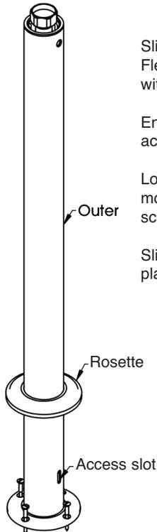
Slide outer tube over the Supply Flex with the Access Slot aligned with stop valve screw.
