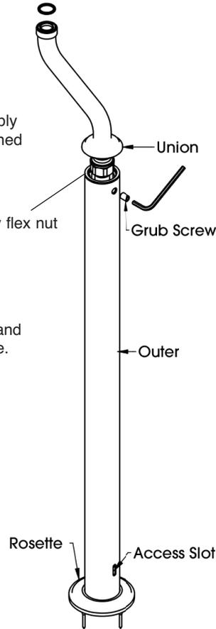
Holding the nut on supply flex, thread on the union. Avoid twisting supply flex.
