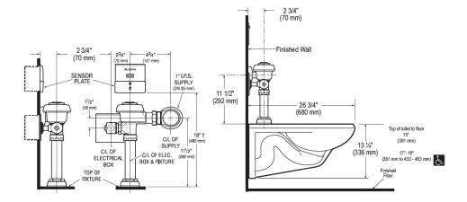
**NOTE**: All vitreous china dimensions shown in these drawings are nominal. Dimensions can vary within the tolerances established in the governing ASME A112.19.2/CSA B45.1 standard. Please take this into consideration when planning rough-in and plumbing layouts.
