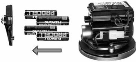
2. Disconnect the white plastic connector that connects the black and red wires on the side of the module.
