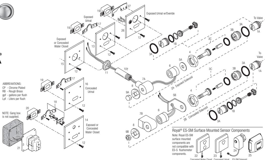
**SOLENOID/SENSOR PARTS AND ASSEMBLIES LIST**
