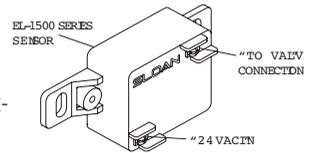
**NOTE: If the 24 volt power supply is ever interrupted for longer than twenty (20) seconds, the start-up mode automatically begins when power is restored.**
