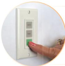
**One Touch** adjustment with a User Switch 479 makes changing between occupied, unoccupied & away temperatures easy for any homeowner.
