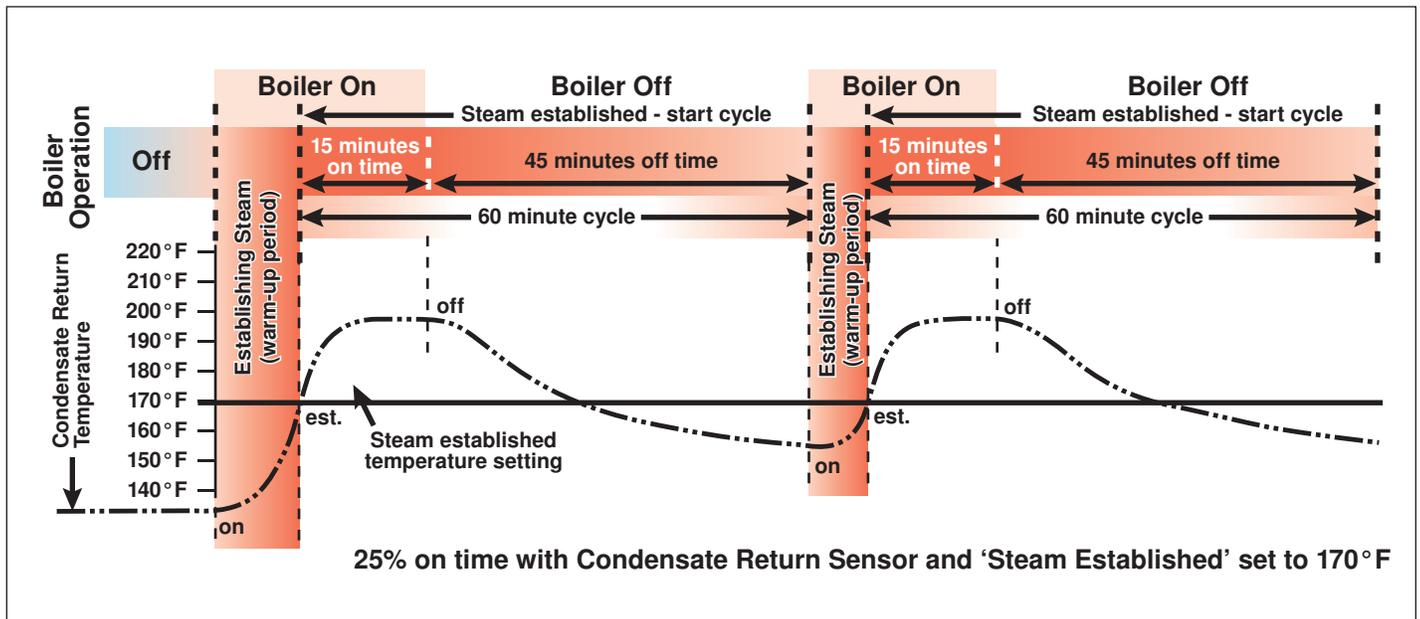
Outdoor reset is a method of operating a heating system based on the fact that the rate at which a building loses heat to the outdoor environment is mostly dependent on the surrounding outdoor air temperature. As the outdoor temperature gets colder, the heat loss of the building increases at a proportional rate. This relationship between heat loss and colder outdoor temperatures is called a heating curve.
