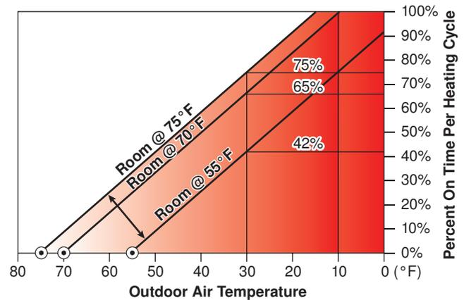
When an indoor sensor(s) is connected to the control, the Room setting becomes a Room Target temperature. The control measures the current air temperature in the room using the indoor sensors. The control then automatically shifts the heating curve so that the measured room temperature reaches the Room Target temperature.
