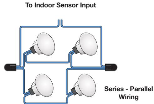
When using two indoor sensor inputs, the control can operate either based upon an average of the two temperature measurements or the control can operate on the lowest of the two temperature measurements.
