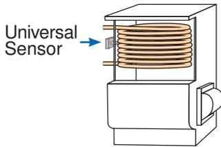
The advantage of using the DHW Tankless Coil feature is that the control can be programmed to operate the tankless coil on a night setback schedule. This can lower fuel usage for domestic hot water heating. The DHW tankless coil operation of the boiler is separate from the steam heating operation and is not affected by the heating system settings.
