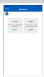
Each building is displayed on the screen as a tile with the building name, address and status. If there are no active errors the status is Ok ✓. When an error condition is present, an Alert ▲ is displayed.
