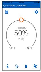
• Click the water drop **b** button to adjust the humidity min and max settings (only available on select thermostat models).
