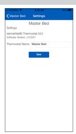
• Click the # button to view the thermostat model, tekmarNet address and change the thermostat name. The name is limited to 16 characters.
