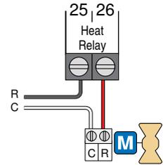
If the heat relay is wired to an electrical contactor:
