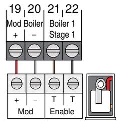
The 4 to 20 mA output can be converted to a 0 - 135  $\Omega$  output for a Modutrol IV™ gas valve actuating motor using a 0 - 135  $\Omega$  tekmar Converter 005 (sold separately).
