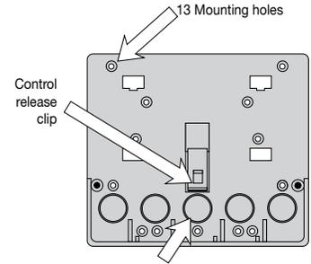
There are 10 conduit knock-outs at the back and bottom of the wiring chamber.
