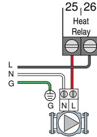
If the heat relay is wired to a 24 V(ac) on-off valve:
