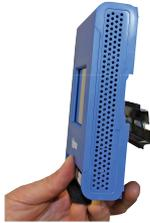
Snap the enclosure onto 35mm DIN rail using the hooks and snaps on the back of the enclosure.
