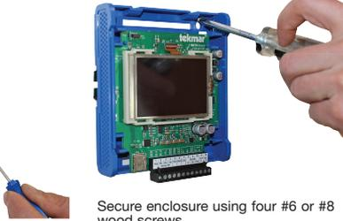
Secure enclosure using four #6 or #8 wood screws.
