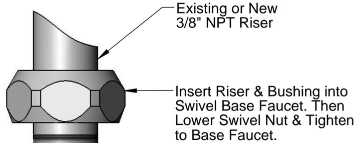
Screw Bushing onto Bottom of Riser w/ LocTite Provided
