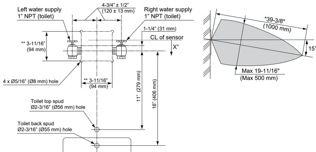
\* X", ± = At least 5" clearance from sensor to tip of toilet seat up position or to top of grab bar is required to avoid false detection.
