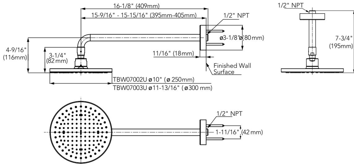
Note: The unit of above dimension is inch (mm).
