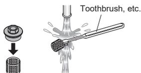
7. Install the water supply filter to the cap, then tighten the cap with the opening/closing tool.
