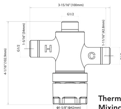
Thermostatic Mixing Valve (TLT20)
