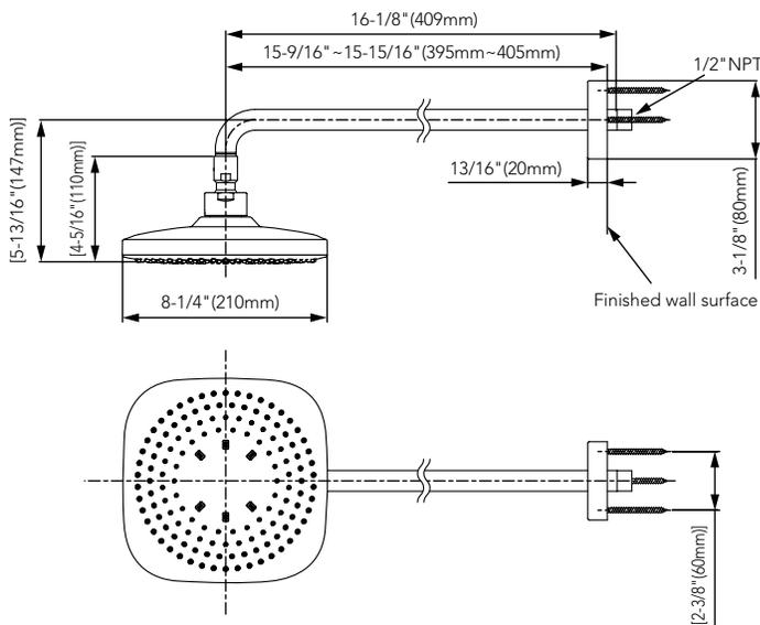
Note: The unit of above dimension is inch (mm); the dimension in [ ] is for reference only. Shower arm and mounting bracket are not included.
