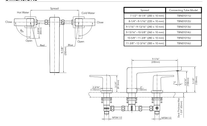
NOTE: Unit for dimensions = inches Dimension in () is mm. Tub filler rough-in sold separately.
