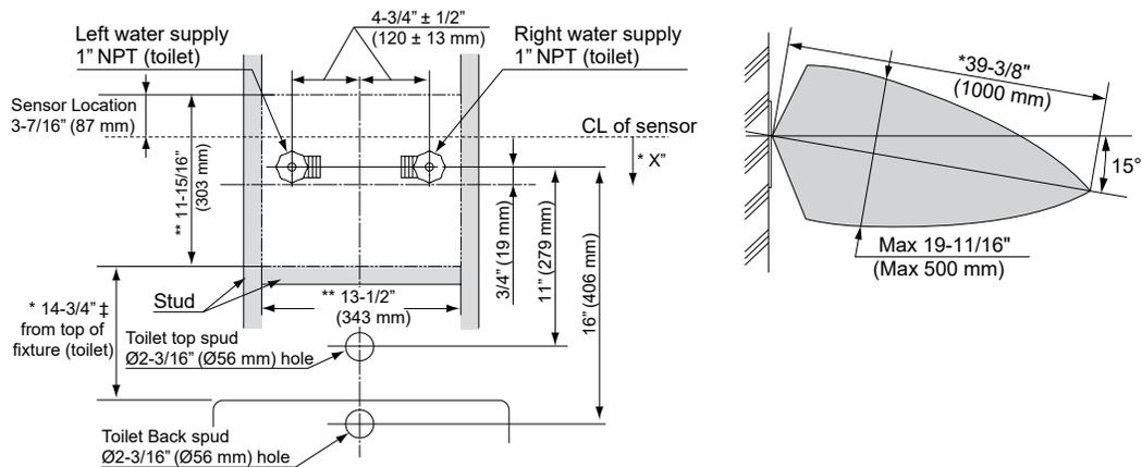
\* X", ± = At least 5" clearance from sensor to tip of toilet seat up position or to top of grab bar is required to avoid false detection.
