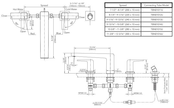
NOTE: Unit for dimensions = inches Dimension in ( ) is mm.
