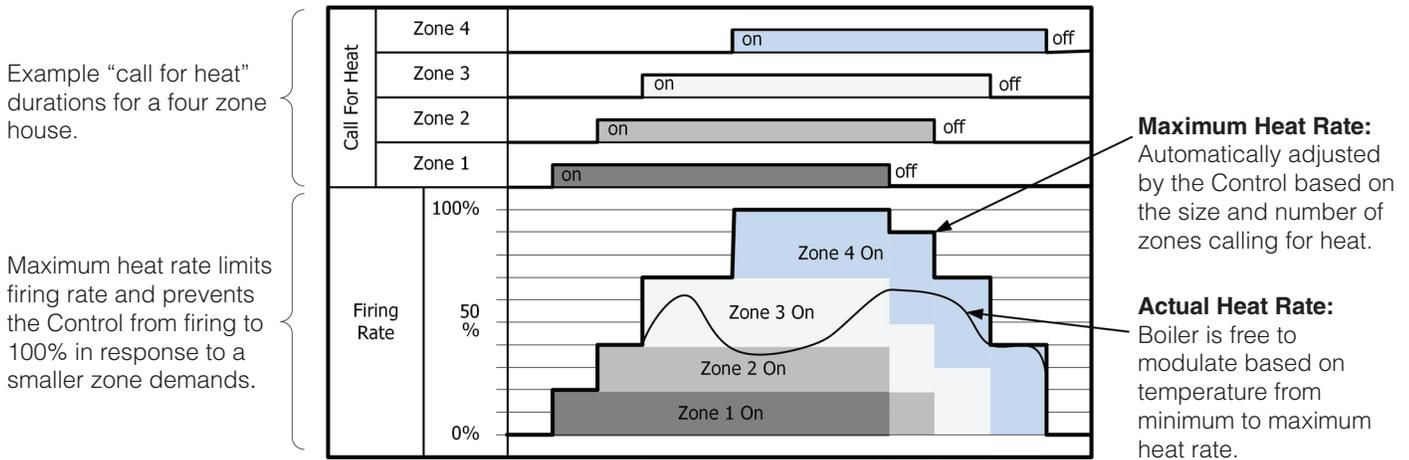
Figure 43: Four Zone House (with Zone Control Connected)
