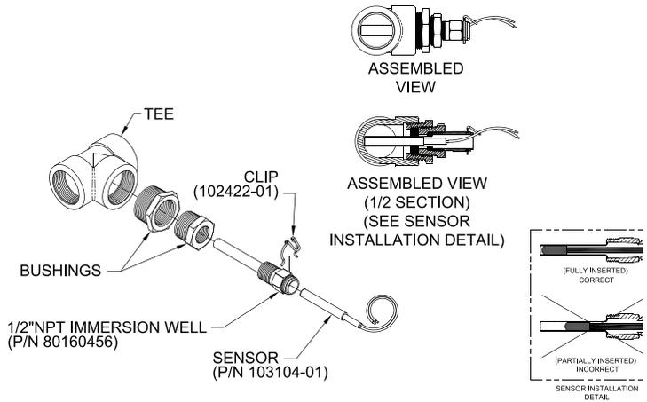
**Figure 32: Recommended “Immersion” Type Header Sensor Installation Detail**
