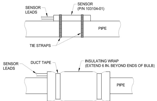
**Note:** The “Strap-On” type sensor must be mounted to the top side of a horizontal section of pipe as indicated in Figures 24A and 25A.
