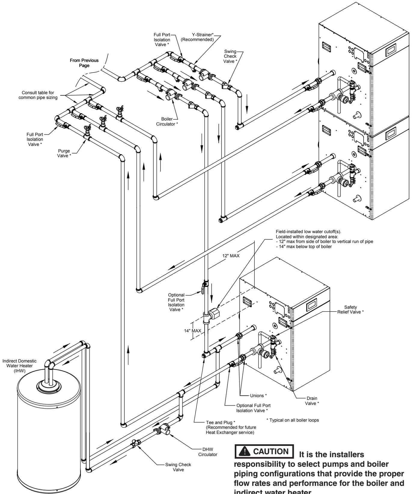
Figure 25B: Alternate Multiple Boiler Water Piping w/Indirect Domestic Hot Water Heater (Page 2 of 2)
