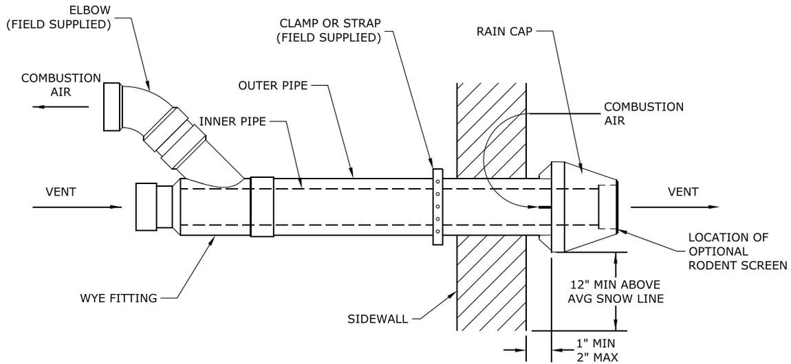
**Figure 6J: Installation of IPEX FGV or DiversiTech CVENT Concentric Terminal thru Sidewall**
