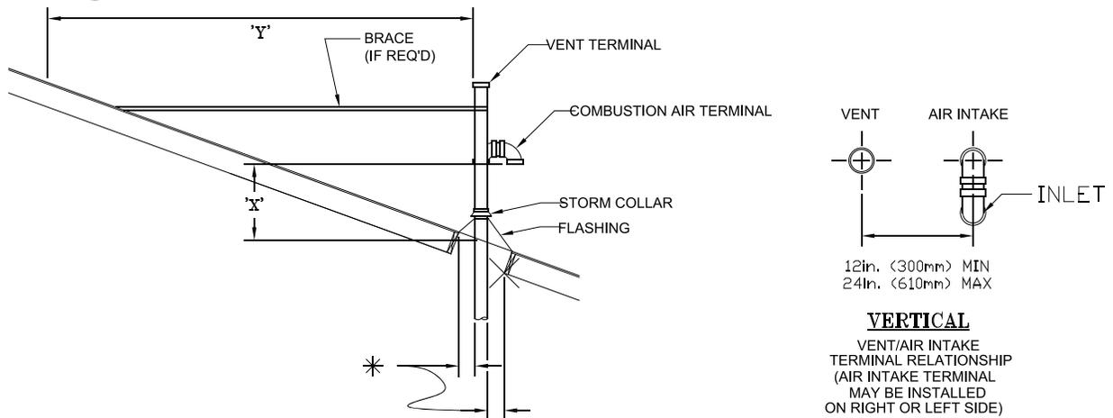
\* VENT PIPE MINIMUM CLEARANCE TO COMBUSTIBLE MATERIAL IS 1in. (25mm). COMBUSTION AIR PIPE MINIMUM CLEARANCE TO COMBUSTIBLE MATERIAL IS ZERO.
