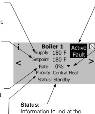
**Figure 41: Boiler Status Screen Detail**
