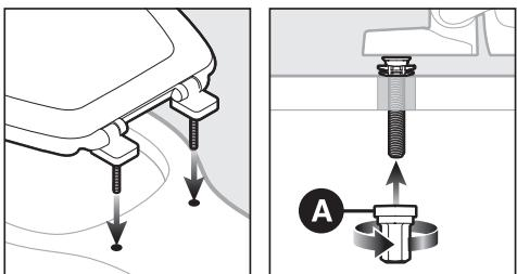
Position sheared off nut directly beneath the side with restricted access bolt hole and as bolt is coming through bolt hole, finger-tighten nut to bolt, pulling it through hole as it is being threaded. Finger-tighten remaining nut on opposite side of bowl.
