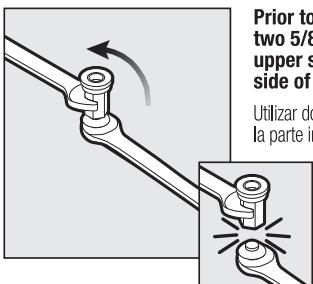
Prior to seat installation, pre-shear off bottom section of (1) nut using two 5/8" wrenches as shown. Discard lower portion of nut, keeping upper section with integrated washer for installation on restricted access side of bowl. Do NOT shear remaining nut at this time.
