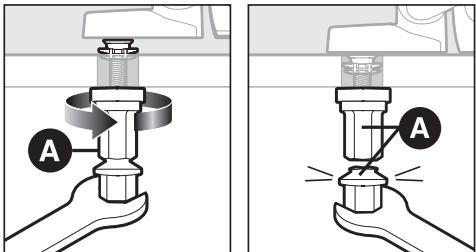
Holding seat centered on bowl, use a 5/8" wrench to tighten unsheared nut until lower portion of nut shears off. Use a 5/8" wrench and tighten pre-sheared off nut 4-5 quarter turns, this will indicate proper tightening torque.
