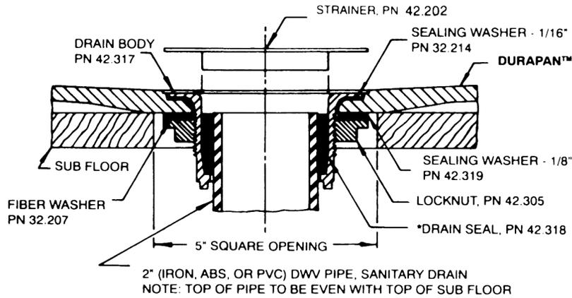
\*AN OPTIONAL DRAIN SEAL, PART NO. 42.320, IS AVAILABLE FOR 2" COPPER (DWV)
