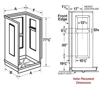
To Determine the approximate Opening for the shower door (enclosure), subtract 2" (5.08 cm) from the shower width. Example: 3248M has a 48" threshold. 48" (121.92 cm) less 2" (5.08 cm) = 46" (116.84 cm). Maximum shower door (enclosure) height can be 72" (182.88 cm).
