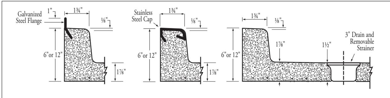
1. Place Mop Receptor on a thin bed of mortar or plaster.
