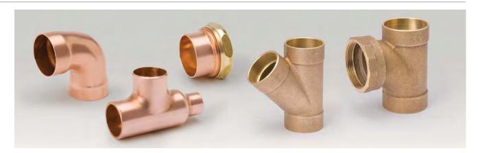
Streamline® Copper Solder-Joint Fittings for DWV plumbing applications are available in both wrot copper and cast bronze materials. Designed for use in non-pressurized sanitary systems, these fittings commonly feature shorter solder cup designs and more sweeping turns. They are available in a wide range of diameters, styles and connections to meet most all sanitary system applications.
