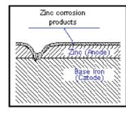
creates additional protection against zinc hydroxide. This cathodic protection prevents corrosion to exposed parts, due to any discontinuity or mechanical damage on the coating.
