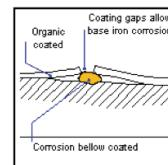
Cathodic iron protection, provided by the metallic zinc coating, is factually based on corrosion being an electro-chemical process.
