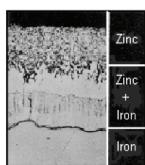
Zinc resists the environment's corrosive actions. Opposite to this, most of the organic coatings (paintings) are environmentally unstable and need to be renewed frequently. When a little failure occurs, corrosion starts and it begins to become larger under the protective coating.
