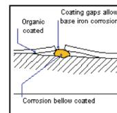
Cathodic iron protection, provided by the metallic zinc coating, is factually based on corrosion being an electro-chemical process.
