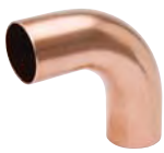
90° Elbow • Long Radius FTG x FTG Wrot Style #: WE-506L
