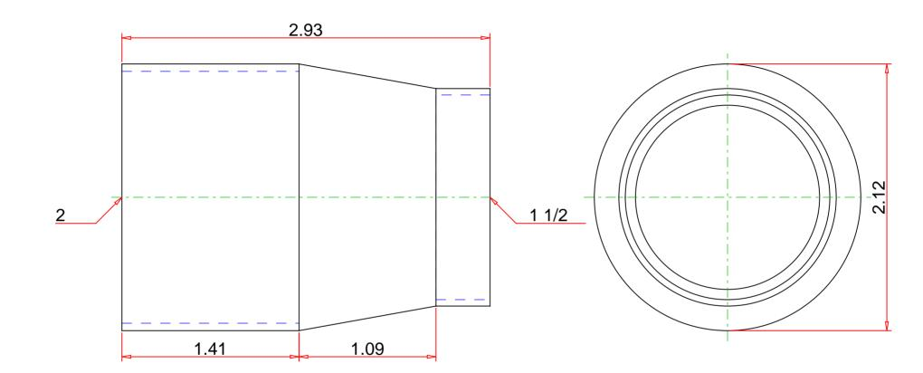
Note: - Drawing not to Scale DISCLAIMER: DIMENSIONS ARE APPROXIMATE AND ARE SUBJECT TO CHANGE WITHOUT NOTICE. ALL ASME DIMS ARE MINIMUM UNLESS NOTED. LAY LENGTH DIMS ARE  $\pm~0.06$ ALL OTHER DIMS ARE NOMINAL. ALL DIMS ARE IN INCHES.
