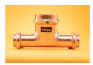
Viega ProPress may only be pressed onto copper tube in accordance with ASTM B88 or B75. When pressing onto B88 copper tube, types K, L, and M may be used. Tempers O60 and O50, known as "soft
