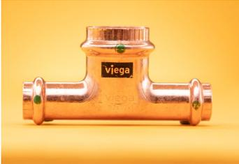
Viega ProPress may only be pressed onto copper tube in accordance with ASTM B88 or B75. When pressing onto B88 copper tube, types K, L, and M may be used. Tempers O60 and O50, known as “soft copper”, are limited to nominal sizes ½" to 1¼". Temper H58, known as “hard copper”, may be used with nominal sizes ½" to 4".
