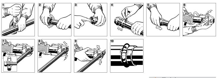
Viega ProPress 1/2" to 2" Fittings For Hard Copper Tubing in 1/2" to 2" and Soft Copper Tubing in 1/2" to 11/4".
