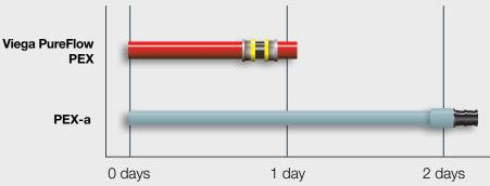
\*Because they pressure test immediately; they don't require time for drying, curing or contracting
