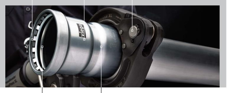
Sealing elements: FKM standard on 304 stainless fittings. MegaPress 316 available with either an FKM or EPDM sealing element. Smart Connect® technology helps easily identify unpressed connections during pressure testing.
