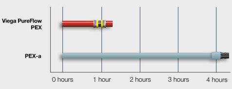
\*Because they pressure test immediately; they don't require time for drying, curing or contracting. Assumes 500-600 fittings, PEX-a connections will take 3 hours longer over the course of the job.
