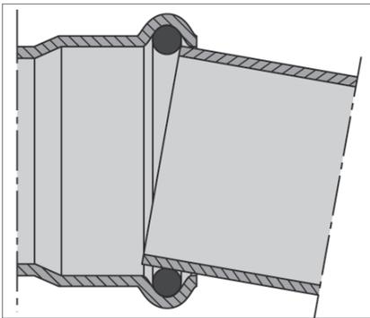
Fittings that do not have cylindrical guides risk making an unsecured connection. Without the guides, installers may damage the sealing element.
