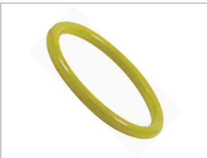
ProPress press fittings may be changed from the factory-installed EPDM sealing element to a yellow HNBR (Hydrogenated Nitrile Butadiene Rubber) sealing element. See [Changing Sealing Elements Product Instructions](#). The HNBR sealing element is used mainly for inert gas, liquid fuel, and lubricant oil. It is commonly used in fuel oil heating systems.
