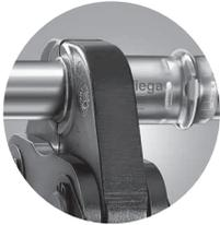
**2** Upon identification, use the press tool to press the fitting, making a secure leak-proof connection.
