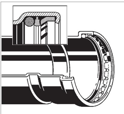
Illustration demonstrates proper fit of grip ring, separator ring, and sealing element.
