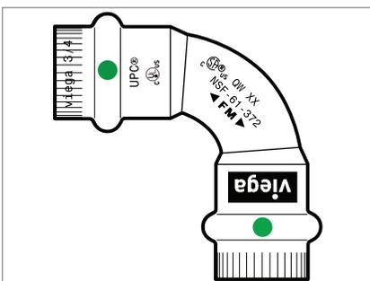
Each ProPress fitting is marked with the following:
