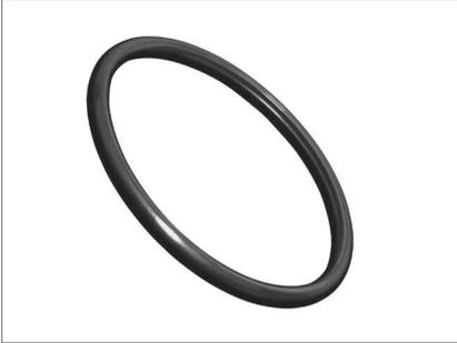
Viega ProPress fittings are manufactured with a high-quality, shiny black EPDM sealing element installed at the factory. EPDM (Ethylene Propylene Diene Monomer) is a synthetically manufactured and peroxidically cured all purpose elastomer. The molded sealing lips also seal tube surfaces with slightly uneven surfaces. Sealing elements are inserted into the fitting using a H1 food grade lubricant registered with NSF and the USDA, and is approved for use under FDA 21 CFR.
