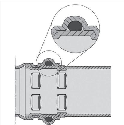
Fittings are radially pressed around the sealing element in a single step.
