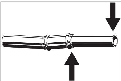
The pressing process can cause deflection (angular misalignment) to occur. When pressing Viega ProPress fittings in a system, the deformation of the fitting is constant. This allows for a consistent leak-free joint every time and is a result of the pressing technique.
