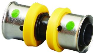
Viega PureFlow Press fittings are available in zero lead bronze and polymer and include a factory-assembled, stainless steel sleeve with three viewing holes and a tool
