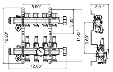
\* When extending the manifold, Viega requires using thread sealant paste on the 1" NPT manifold end connection.
