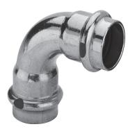
Viega ProPress fittings are for use with type K, L and M hard copper tubing from 1/2" to 4" and soft copper tubing in ½" to 1¼" diameters. All tubing must comply with the ASTM B88 standard.
