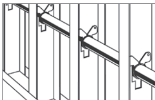
Suspension clip fasteners used to protect tubing from abrasion when passing through steel studs
