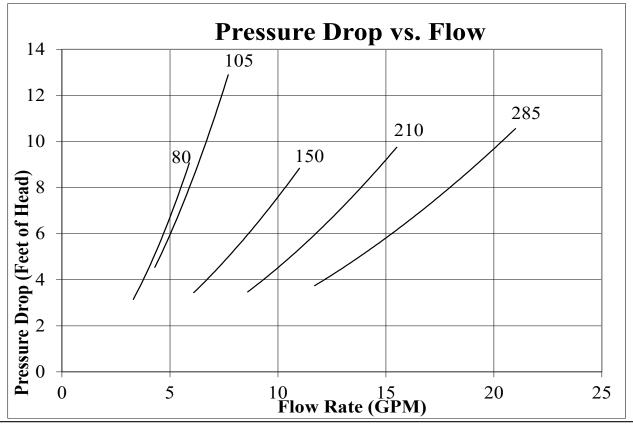
Table 6-3: Recommended Circulators for 50 ft. Equivalent ft. Near Boiler Piping [Approximately 20 ft. Straight Pipe, (4) 90° Elbows, and (2) Full Port Ball Valves]
