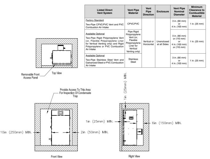
Figure 3-1: Clearances To Combustible and Non-combustible Material, Floor Standing
