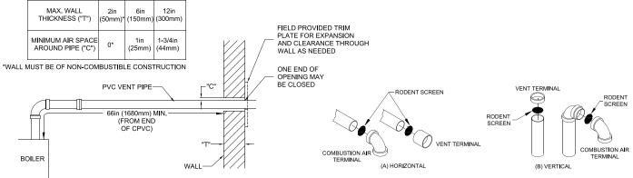
Figure 4-32: Wall Penetration Clearances for PVC Vent Pipe
