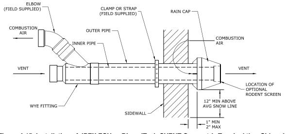
Figure 4-15: Installation of IPEX FGV or DiversiTech CVENT Concentric Terminal thru Sidewall
