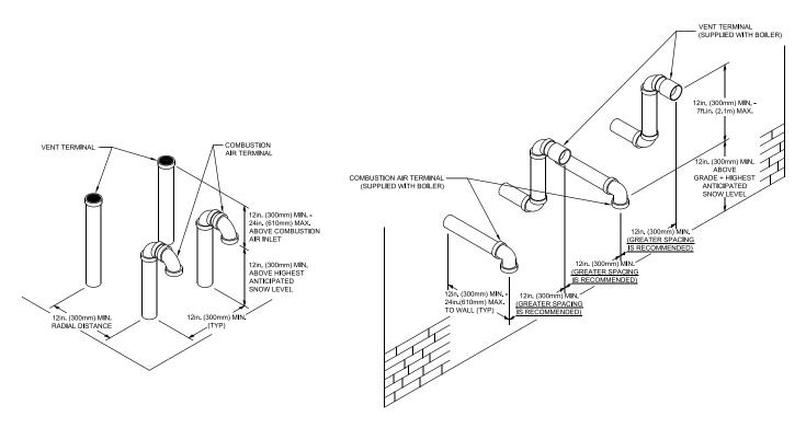
Figure 4-49: Multiple Boiler Direct Vent and Air Intake Terminations
