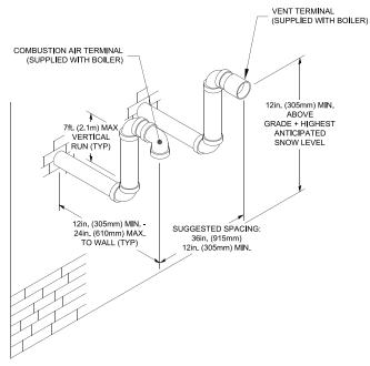
Figure 4-7: Direct Vent - Snorkel Vent and Air Intake Horizontal Sidewall Terminations
