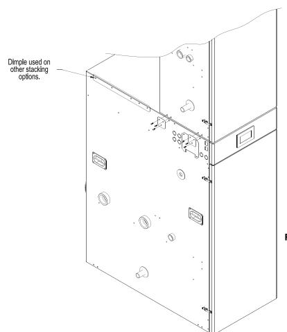
Figure 3-7: Stacking Boiler Attachment Bracket Placement
