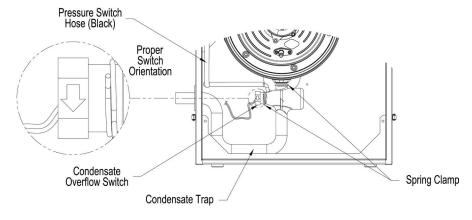
Figure 11-2: Condensate Overflow Switch Orientation
