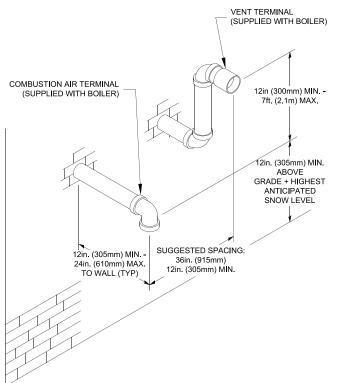
Figure 4-8: Direct Vent - Staggered Vent and Air Intake Horizontal Sidewall Terminations
