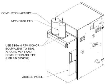
Figure 4-22: Field Installation of CPVC Vent Pipe - Wall Mounted Boiler Builds
