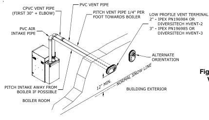
Figure 4-10: Direct Vent - Horizontal Two-pipe Venting/Air Intake with IPEX Low Profile or DiversiTech HVENT Terminal
