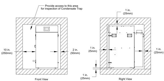
Figure 3-2: Clearances To Combustible and Non-combustible Material, Wall Mounted
