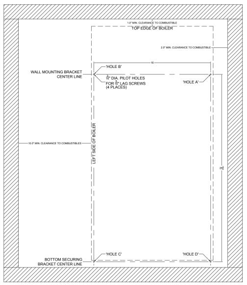
Figure 3-3: Wall Mounting Hole Location / Layout
