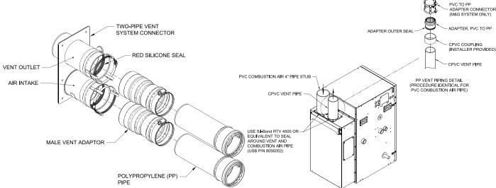
Figure 4-34: Vent System Field Modification to Install PVC to PP Adapter (M&G/DuraVent shown)
