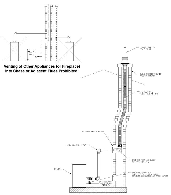
Figure 4-36: Flexible PP Vent in UNUSED Masonry Chimney with Separate Combustion Air Intake
