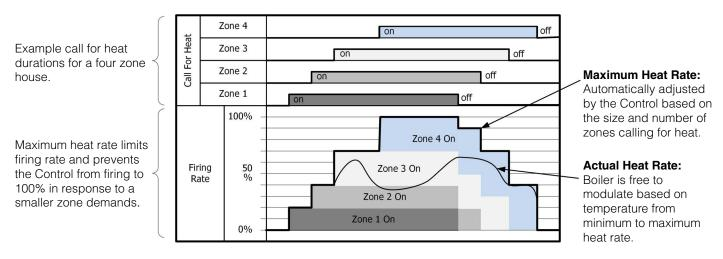
Figure 10-10: Four Zone House (with Zone Control Connected)
