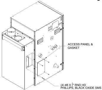
Figure 3-5: Access Panel and Gasket Installation
