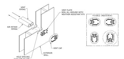
Figure 4-12: Installation of DiversiTech HVENT Terminal thru Sidewall
