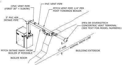
Figure 4-13: Direct Vent - Horizontal Two-pipe Venting/Air Intake with IPEX FGV or DiversiTech CVENT Concentric Terminal
