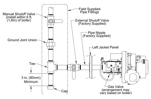
Figure 7-6: Recommended Gas Piping
