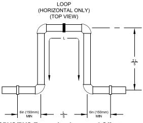
Figure 4-24: CPVC/PVC Expansion Loop and Offset
