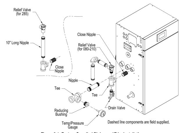
Figure 6-1: Factory Supplied Piping and Trim Installation
