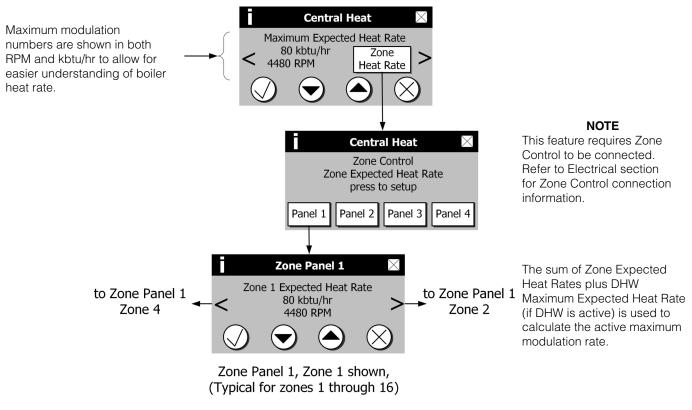
Figure 10-11: Expected Heat Rate Adjustment (with Zone Control Connected)
