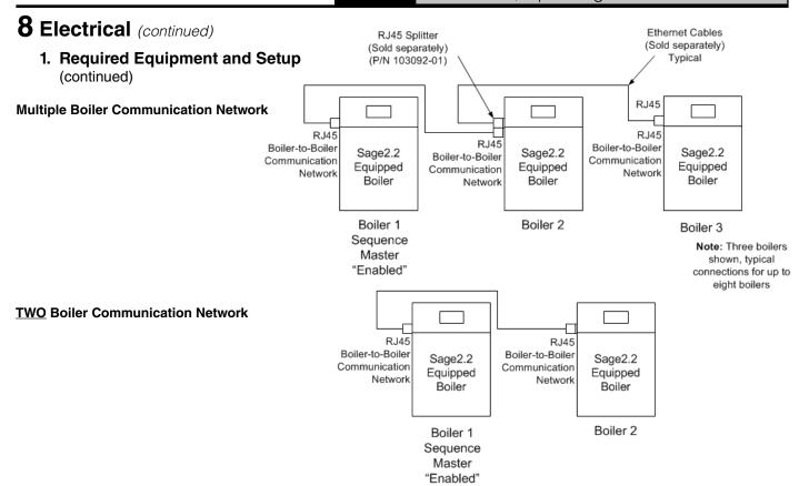
Figure 8-13: RJ45 Splitter Installation Detail
