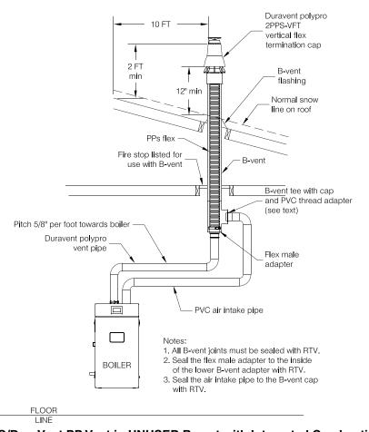
Figure 4-38: Flexible M&G/DuraVent PP Vent in UNUSED B-vent with Integrated Combustion Air Intake
