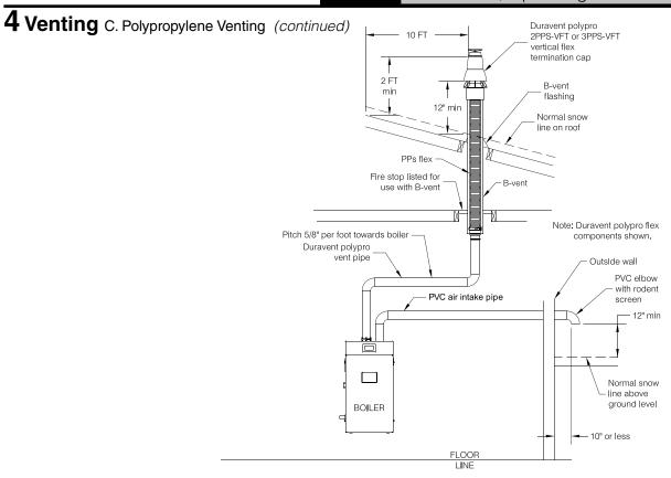
Figure 4-37: Flexible PP Vent in UNUSED B-vent with Separate Combustion Air Intake
