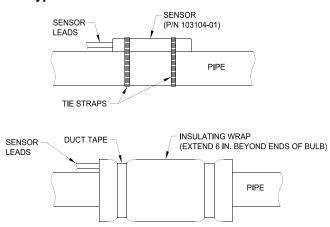
**Note:** The "Strap-On" type sensor must be mounted to the top side of a horizontal section of pipe as indicated in Figures 6-9 and 6-11.
