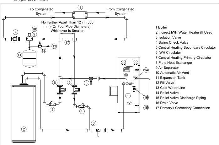
Figure 6-8: Isolation of the Boiler From Oxygenated Water with A Plate Heat Exchanger
