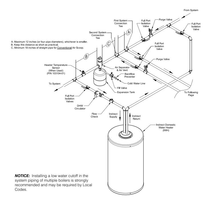
Figure 6-9: Multiple Boiler Water Piping w/Domestic Hot Water Heater (Page 1 of 2)
