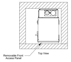
c. 5/16 in. x 2 in. lag screws and 5/16 in. plated washers are intended for mounting the boiler directly onto studs covered with ½ in. drywall. When the boiler is attached to other types of construction, such as masonry, use fasteners capable of supporting the weight of the boiler and attached piping in accordance with good construction practice and applicable local codes.
