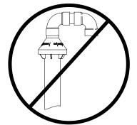
Figure 9-8: Do Not Install U-bend or any other Fittings on Terminal Rain Cap
