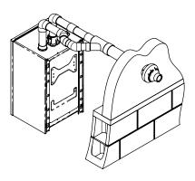
Figure 7-3: Sidewall Concentric Termination see Section 8 for details
