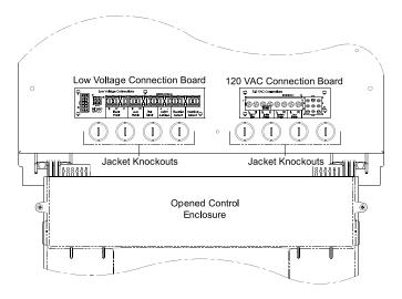
Figure 12-1: Location 120 VAC and Low Voltage Connection Boards
