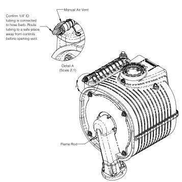
Figure 14-1: Manual Air Vent Location
