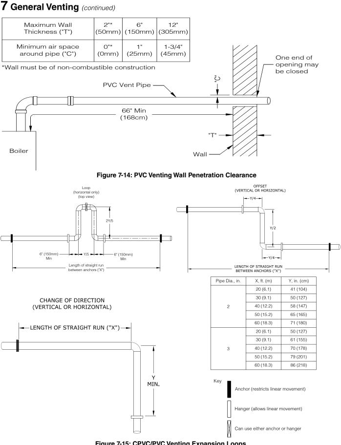
Figure 7-15: CPVC/PVC Venting Expansion Loops
