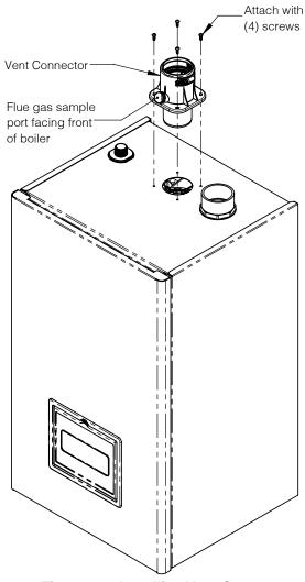
Figure 6-2: Installing Vent Connector
