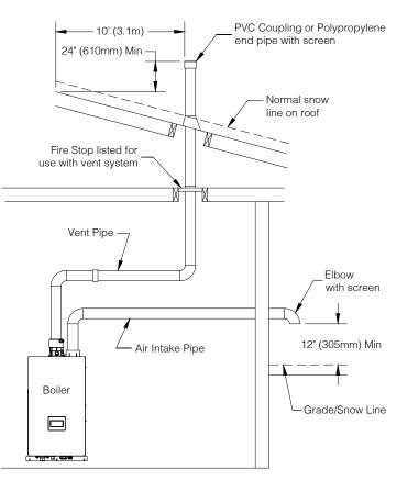
Figure 9-5: Alternate Vertical Vent/Sidewall Air Terminal
