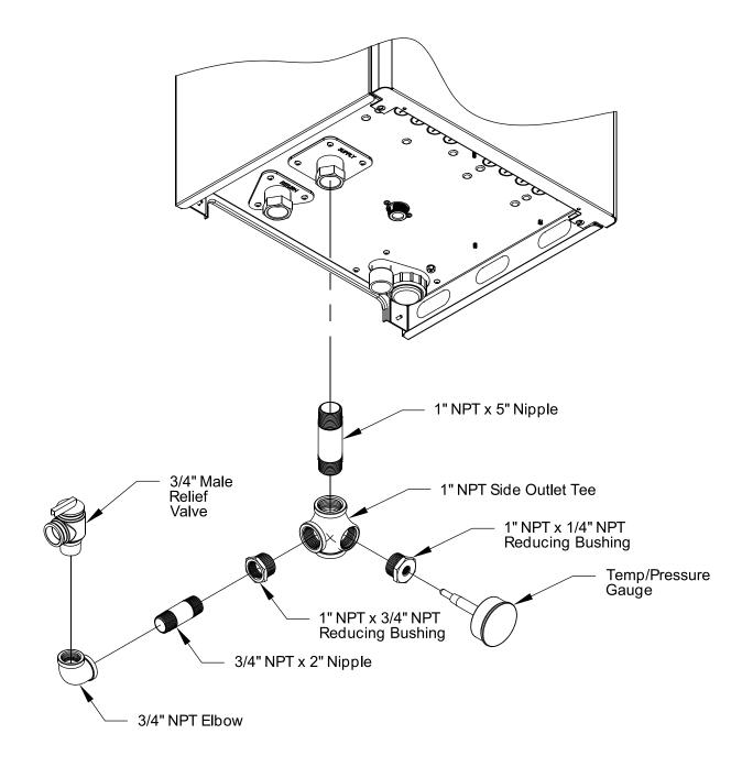
Figure 10-5: Near Boiler Piping Supplied with Boiler
