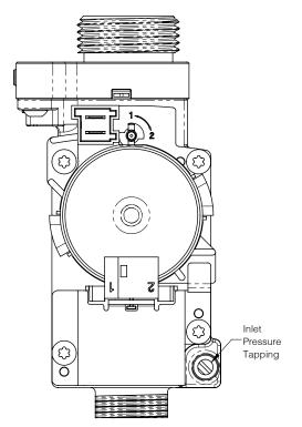
Figure 14-8: Gas Valve Inlet Pressure Tap
