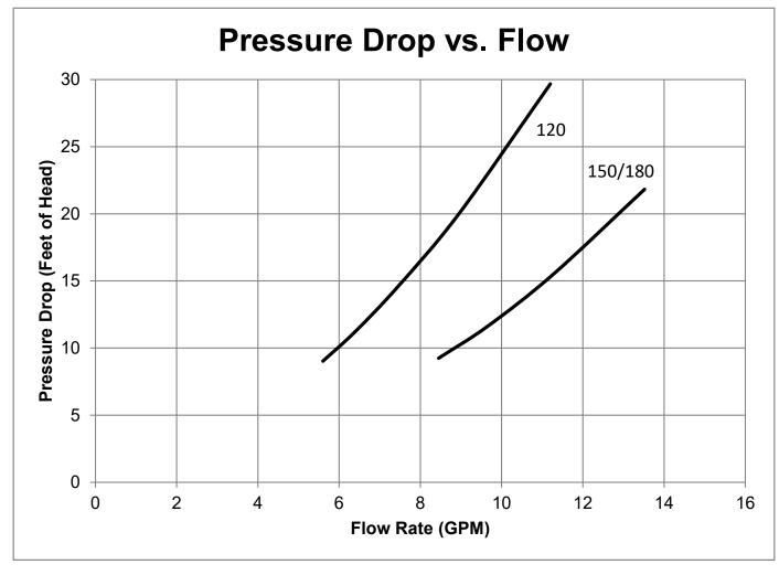
Figure 10-2: System Curve w/ 50 Equivalent ft. of Piping
