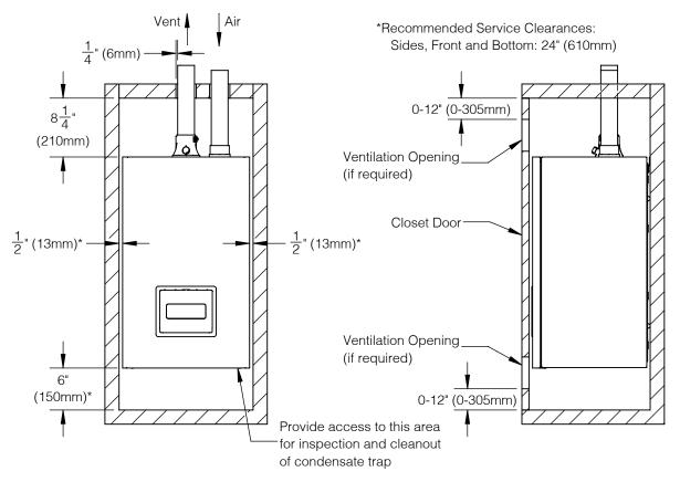
Figure 5-1 : Minimum Clearances to Combustible Construction
