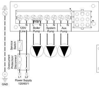
Figure 12-2: 120 VAC Connections
