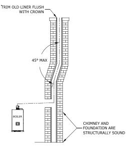
Figure 9-17: Masonry Chimney Chase Requirements
