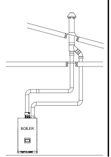
Figure 7-5: Vertical Concentric Termination - see Section 9 for details
