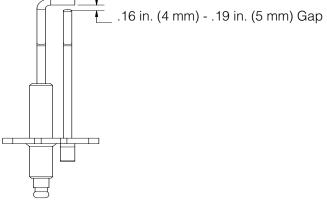
Figure 17-2: Ignitor/Flame Sensor Spark Gap
