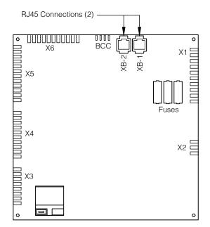
Figure 12-4: Boiler-to-Boiler Connections
