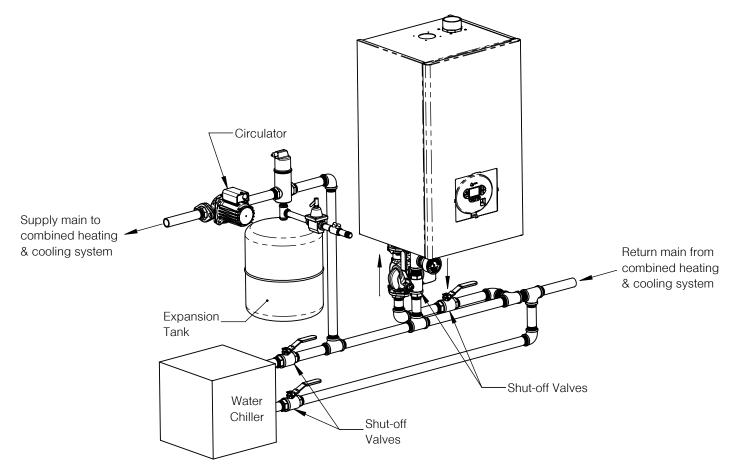
Figure A-1: Isolated Boiler from Refrigeration System
