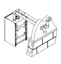
Figure 7-1: Sidewall Termination with Fittings see Section 8 for details
