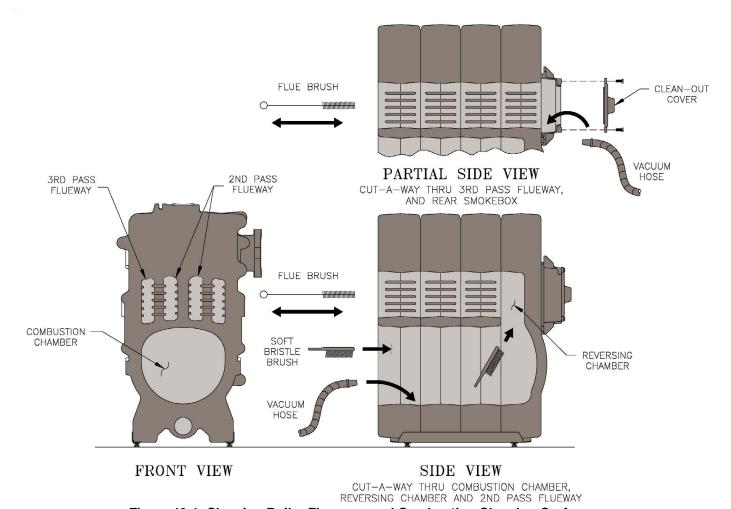
Figure 10-1: Cleaning Boiler Flueways and Combustion Chamber Surfaces
