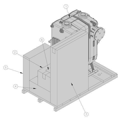
Figure 2-1: MegaSteam™ Unit-Pak Boiler Shipment Contents (outside container removed)
