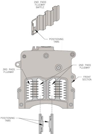
Figure 2-7: Flueway Baffle Positioning/Orientation in Flueways
