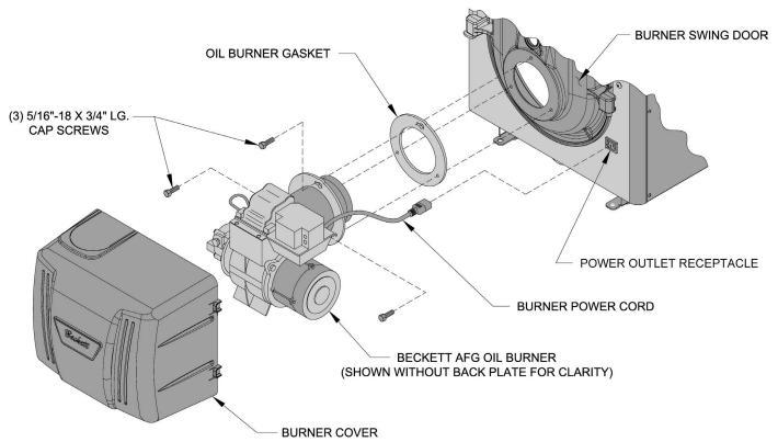
Figure 2-11: Oil Burner Installation (Beckett Burner Shown)
