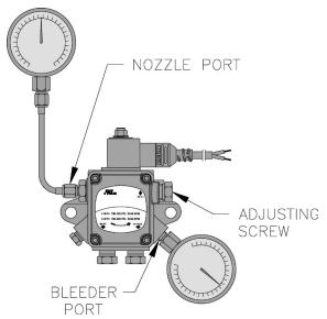
Figure 8-1: Adjusting Fuel Pump Pressure
