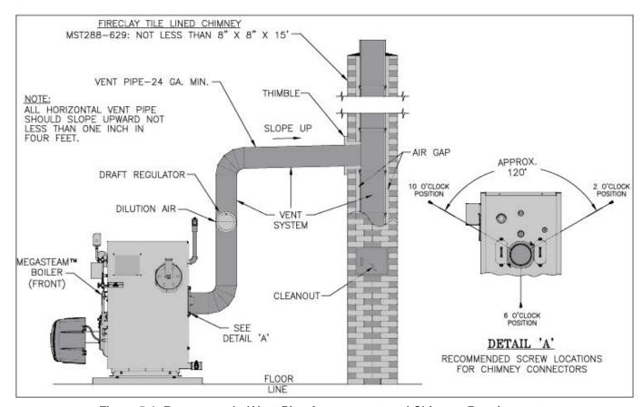
Figure 5-1: Recommended Vent Pipe Arrangement and Chimney Requirements
