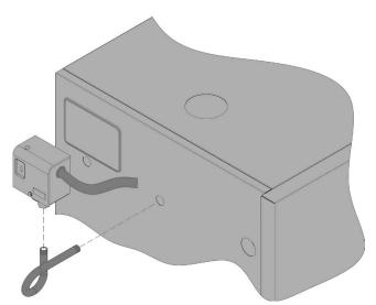
Figure 2-10: Pressure Limit Installation
