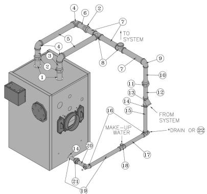
NOTE: Item 14 may need to be installed before the boiler is jacketed.
