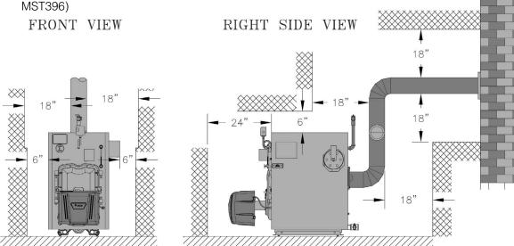
Figure 1-4: Minimum Installation Clearances To Combustible Materials (Inches)
