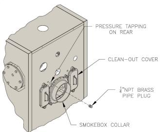
Figure 5-3: Smokebox Pressure Tapping for Checking Draft at Breech
