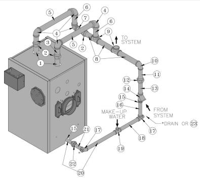
NOTE: Item 15 may need to be installed before the boiler is jacketed.
