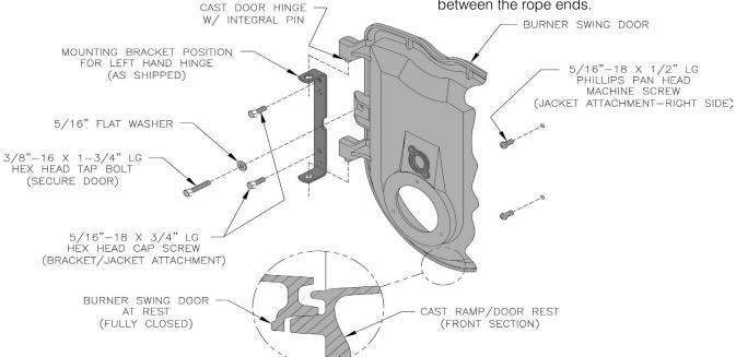
Figure 2-3: Partial Front View - Burner Swing Door Mounted to Boiler - Fully Closed and Secured
