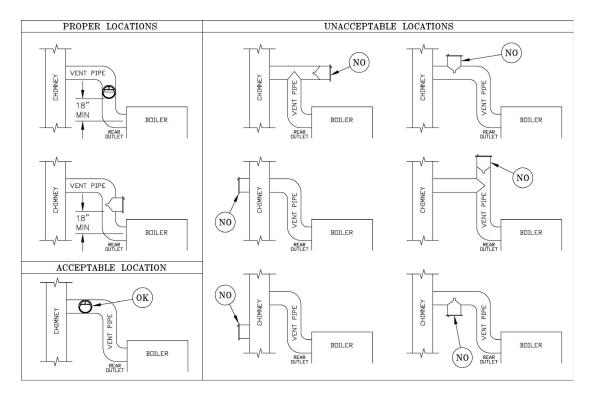
Figure 5-2: Proper and Improper Locations of Draft Regulator
