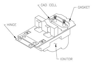
Figure 8-3: Cad Cell Location
