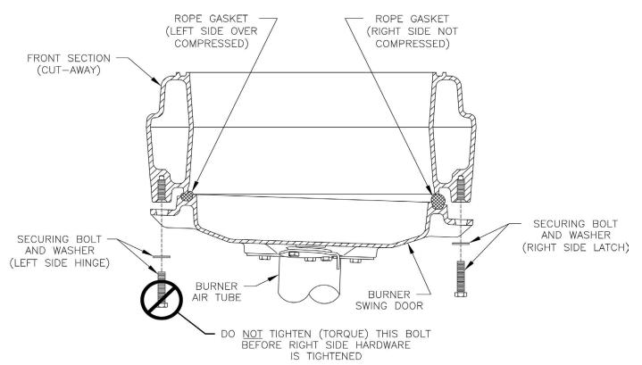
Figure 2-6: Top View - Burner Swing Door Fully Closed but Not Properly Secured or Sealed
