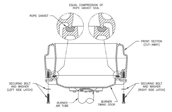
POSITION 1 (PROPERLY CLOSED AND SECURED)
