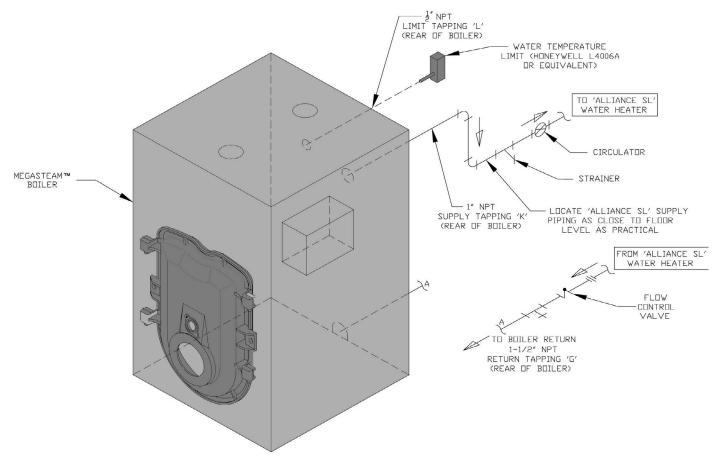
Figure 4-3: Alliance SL™ Water Heater Piping with MegaSteam™ Boiler
