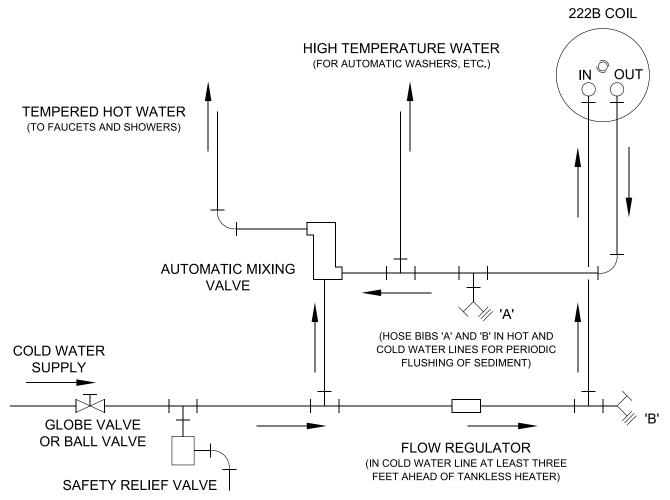
Figure 4-1: Schematic Tankless Water Heater Piping
