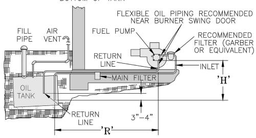
Figure 7-4: Two Pipe Oil Lines
