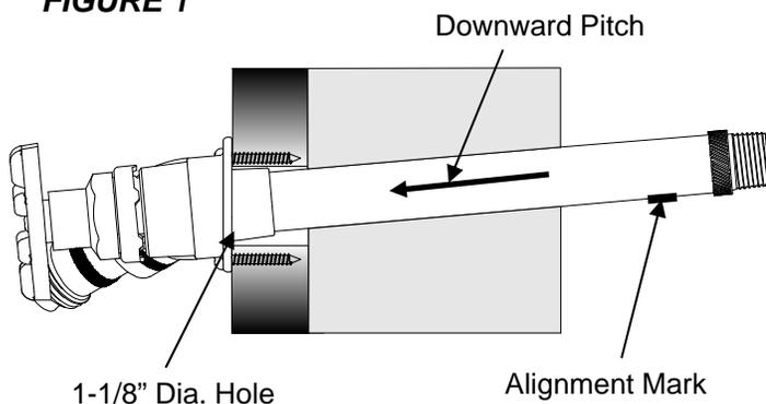
The proper pitch is built into the flange
