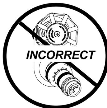
Wall faucets must be properly installed and operated to insure drainage. Improperly installed or operated wall faucets may freeze and burst in freezing weather.
